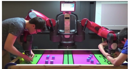
Figure 1: In CS 4752/5752, the students learn robotic manipulation hands-on with Baxter. Instead of a final exam, the students compete in a final competition that shows off the cumulative capabilities they have implemented throughout the semester. The game is similar to soccer, where each team controls one of Baxter's arms to defend their own goal and score on the opponent.
