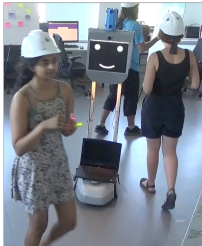
Figure 3: Our socially-competent robot navigates among people by modeling the group’s motion topologically [10, 24–29].
