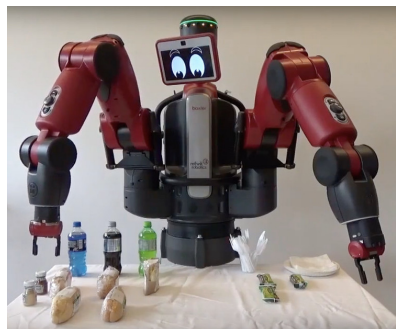
Figure 4: The Baxter Deli system can take verbal orders and serve food to customers. By manipulating success and failure, we use it as a testbed for how people form mental models of robots.
