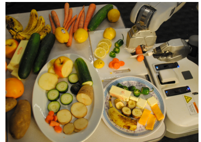
Figure 1: DeepMPC masters the complex dynamics of food cutting by solving the dynamics and control problems separately [8].
